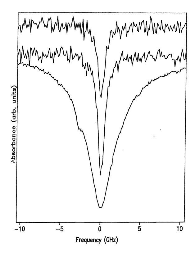
has increased dramatically, ~ 300%. At the same time, the depth of this hole has increased only slightly, ~ 20%. The combination of these two effects demonstrates that the hole has saturated and that additional non-resonant ZPL are being burned via absorption through the tails of the homogeneous absorption lines which overlap the resonant ZPL.
