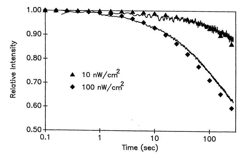
Figure 12: Single frequency scans of the ZPH corresponding to the hole growth curves of Fig. 11. The upper curve has a  $\Delta$ OD of 0.035 corresponding to a 12% hole while the lower trace represents a 38% hole,  $\Delta$ OD = 0.11
