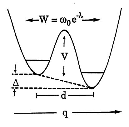
viewed as originating from the corresponding well state of  $TLS_{ext}^{\alpha}$  (not shown). Provided phonon-assisted tunneling is competitive with decay of state  $\beta$ , the asymmetry parameters ( $\Delta$ ) for  $TLS_{ext}^{\beta}$  and  $TLS_{ext}^{\alpha}$  are different (in sign and/or magnitude) and tunneling relaxation in  $TLS_{ext}^{\alpha}$  is slow on the time scale of the experiment, a mechanism for persistent hole production emerges.
